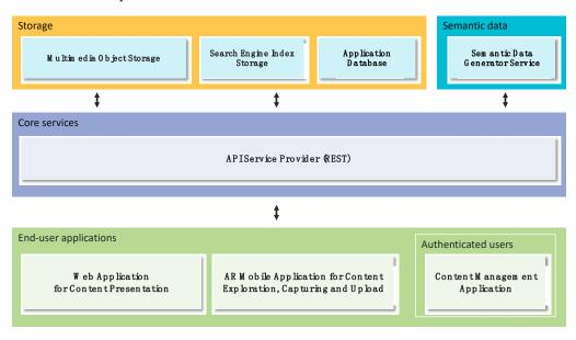
Figure 5. Functional architecture of the InCulture system.
